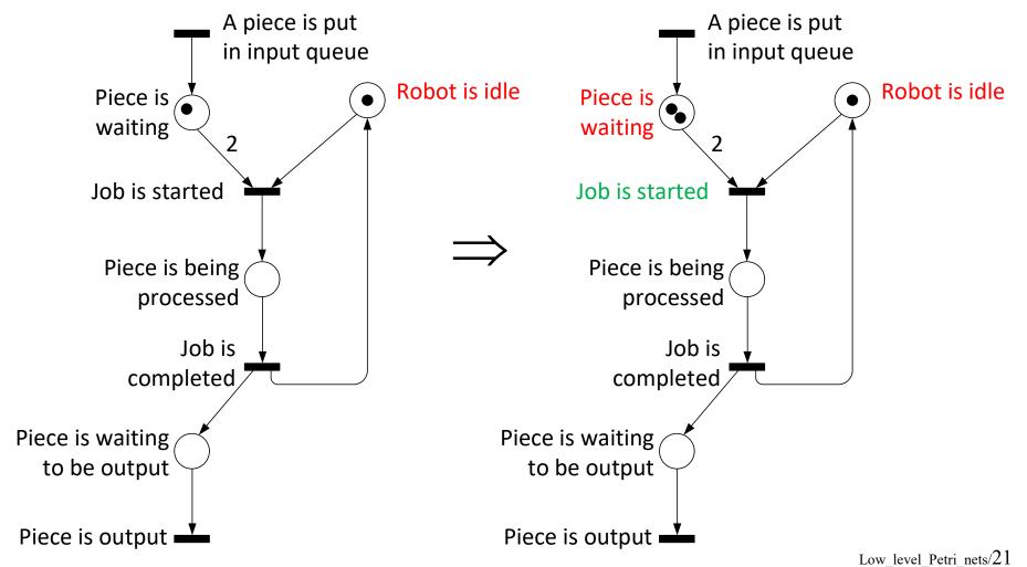
Self-loop: robot is idle until the piece is being processed
